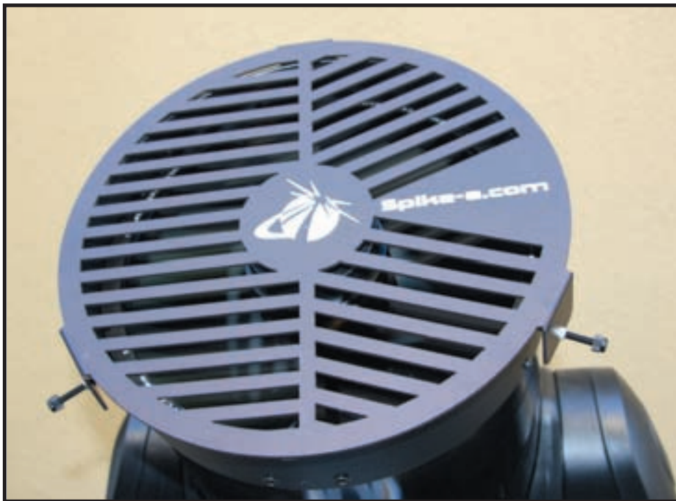
Image 1: Mask mounted on a Celestron CPC 1100 XLT scope. Note the clean machining, anodized finish, and nice non-marring screws used to securely anchor the mask to the scope.
