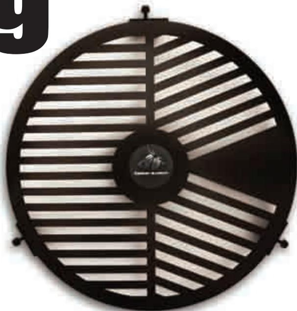
**Image 1 - A Spike-a-brand Bahtinov Mask. It's the relative angles of the groups of slats in the mask which generate the tell-tale spike pattern.**
