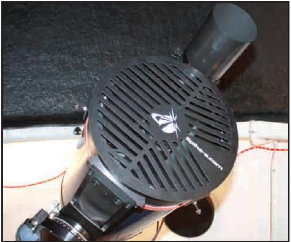
**Image 3 - Always place your mask on your scope in the same orientation. The author aligns his mask so the logo is upright and the center column of aluminum is in line with the counterweight shaft.**
